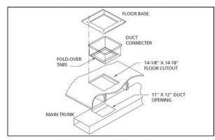
The furnace may be on combustible flooring (expect carpeting) when installed with 86AA001-Duct Connector and 87FB0005 Floor Base.
